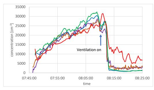
The figure on the left shows the efficiency of the system. With the ventilation initially switched off, aerosol particles are generated by spraying a saline solution. In this measurement, four sensors were placed in the corners of the canopy and one under the canopy roof (red curve).
