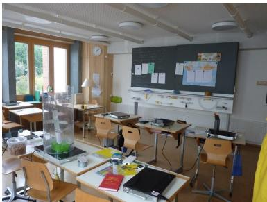
For the aerosol measurements, a source (salt particles by spraying a salt solution) was installed on a desk and a sensor measuring the particle concentration was installed on each desk. Measurements were taken in an empty classroom, with body heat simulated by hot plates, as shown in the picture on the left, but also during class. The results are very similar.
