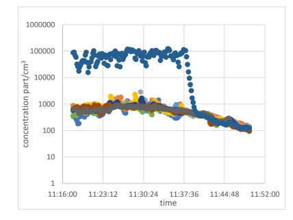
Example of a measurement during class. The blue curve shows the particle concentration at the source, the others show the concentration at the individual desks. It can be seen that the concentration at the desks is about 2 orders of magnitude lower and that this reduction is achieved at all desks.
