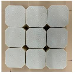
These filters are prefabricated in square blocks (140x140x152 mm) and have an internal surface area of 2.46 m2. Such a unit can be used up to a throughput of about 90m3/h (spatial velocity SV max 10 1/s, face velocity 1 cm/s). Depending on the required flow rate, several such blocks can be glued together to form a larger filter. The illustration shows such a filter block consisting of 9 individual filters as used in a classroom (room volume 140m3).
