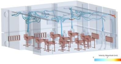
Example of a flow simulation showing that a good vertical flow is achieved.
