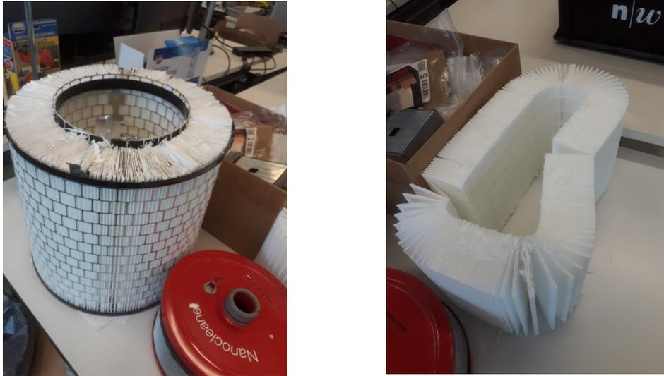
Figure 3: Cut filter
