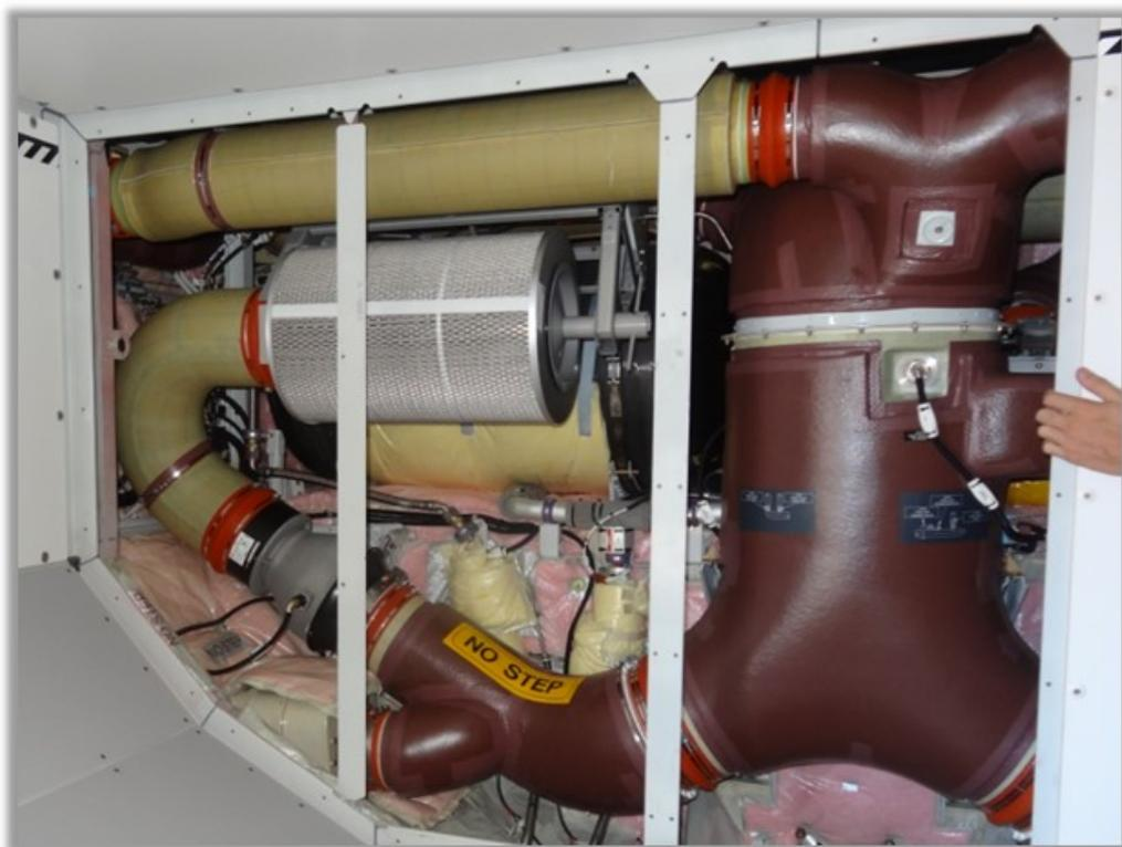
Figure 2: Installation of the filter in the cabin floor
